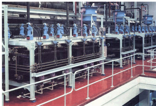
Counter-current mixer-settler equipment: platinum, palladium and iridium are selectively extracted from the aqueous phase by an immiscible organic solvent.
