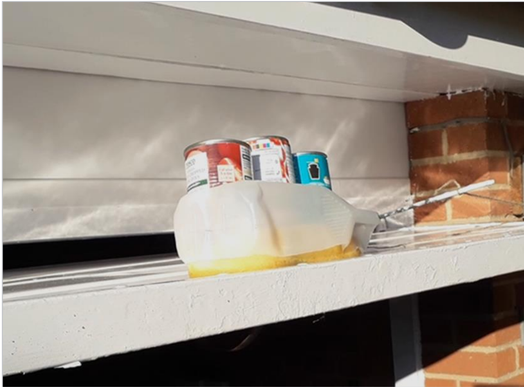
Figure 4 A simple experiment to estimate the drag forces in cleaning a garage door with a wet sponge
