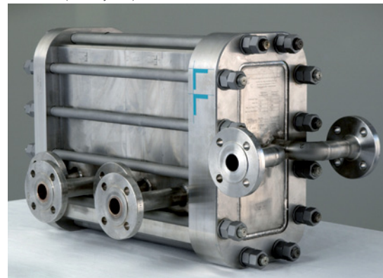
Figure 4: A production-scale microreactor designed by FZK (now KIT). In industrial use, its high heat-transfer capability gives tighter control of reaction conditions, leading to better process performance
