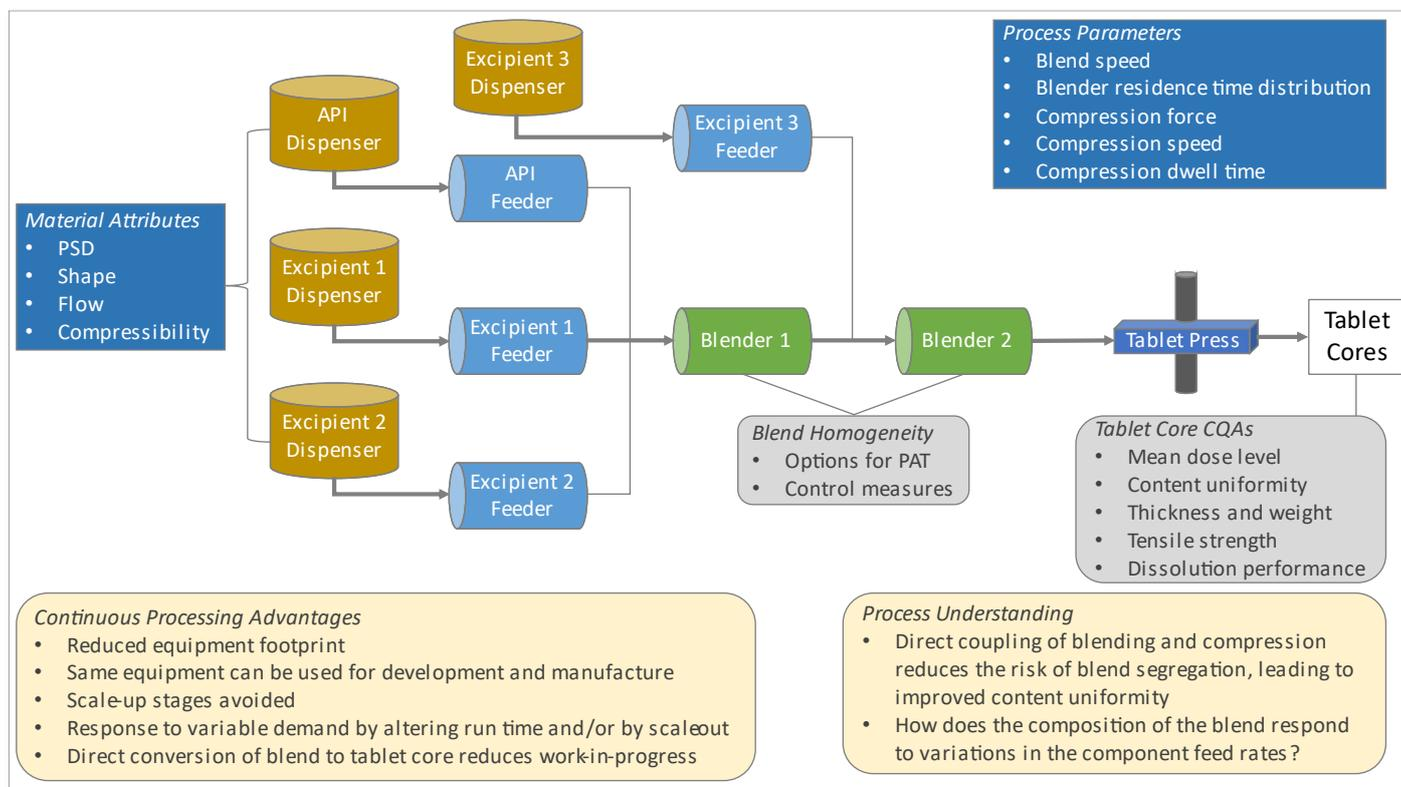
Process Intensification links with Process Understanding to deliver the advantages associated with Continuous Direct Compression of pharmaceutical tablet cores
